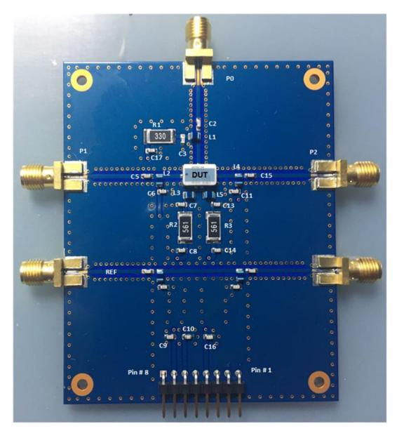
Test Condition 1: P0-P1 Low Loss & P0-P2 ISOLATION
